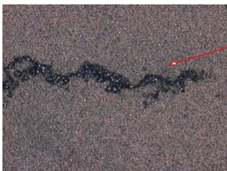
Dielectric Cracks (CRD)
