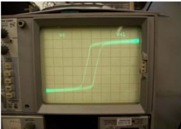
Figure 2. Effect of Thermal Anneal on G113
